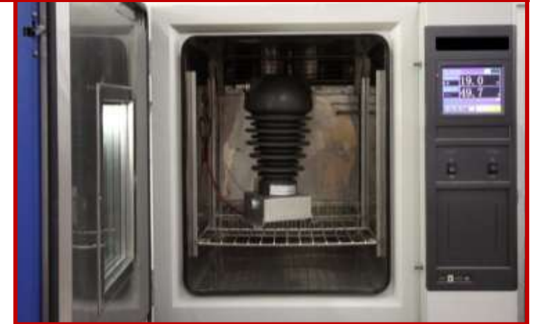
Climatic chamber for the accelerated ageing test through automated duty cycles
